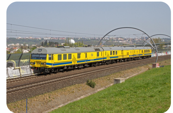
Diagnostic unit for non-destructive track measurement DJ NDT.
